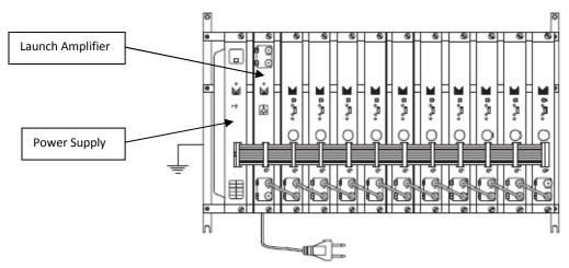
**IMPORTANT:** Layout of the modules must be as shown above. Power Supply (FA-310/312) must be located on the far left hand side and launch amplifier (PA-720) must be the next module in the chain. Please look at the above picture.
