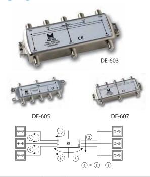
Tap-offs for terrestrial and satellite TV with six tap outputs, covering the 5MHz to 2,300MHz frequencies. They distribute part of the input signal to their tap outputs while the main part of the signal continues to the output. The response of the tap outputs is flat, without equalisation. Available in different tap-off attenuation values.
